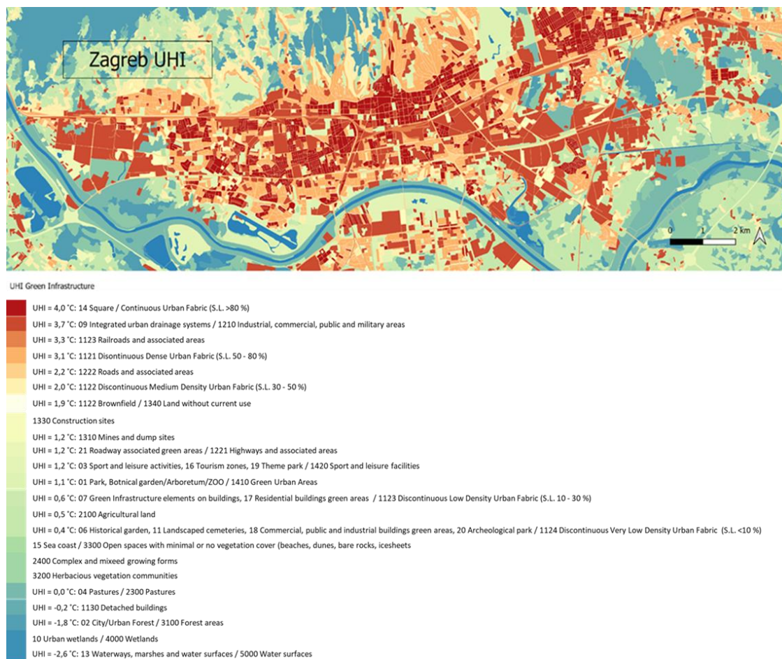
Figure16 Example of a UHI effects map for the City of Zagreb with the associated UHI categories in accordance with the Urban Atlas and the Green Infrastructure Registry
