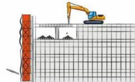
2. Continue demolition of slabs and beams.
